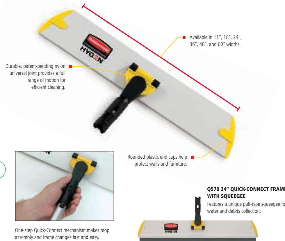
SECURE MOP ATTACHMENT Aluminum frames have removable hook-and-loop strips on the underside for attaching mops. Replaceable strips slide into channels and are held in place by removable end caps.
